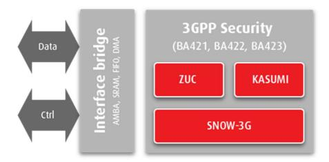
The unique architecture of our 3GPP IP cores enables a high level of flexibility. The throughput and features unique to each application can be taken into account in order to select the most optimal configuration of the implemented IP. The IP cores can achieve a throughput of several tens of Gbps when driven at corresponding frequencies and resource usage.
