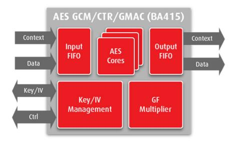
Figure 1: High-speed AES-GCM/CTR/GMAC block diagram
